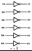
SN5404 . . . J PACKAGE SN54LS04. SN54S04 . . . J OR W PACKAGE SN7404 . . . N PACKAGE SN74LS04. SN74S04 . . . D OR N PACKAGE (TOP VIEW)
